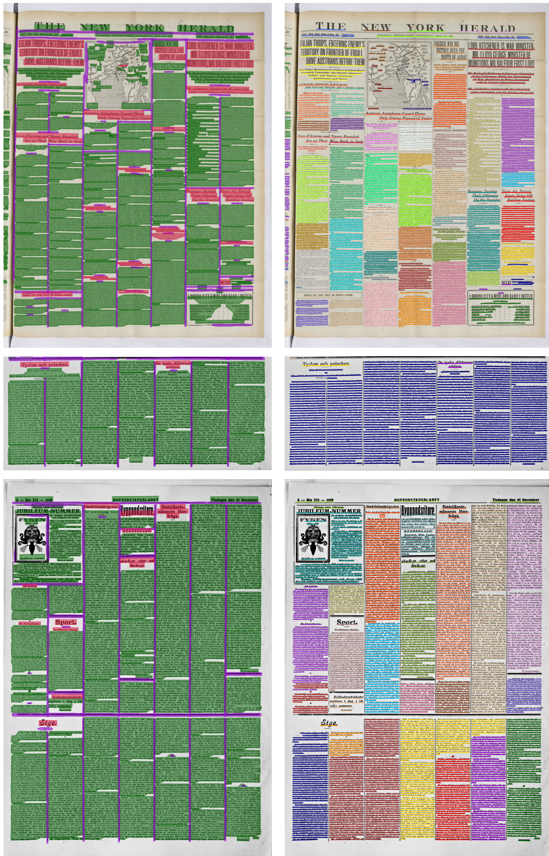
Figure 16: Example outputs for the separator detection, heading detection and text block detection models (left column) and the subsequent AS output of the GNN (right column).
